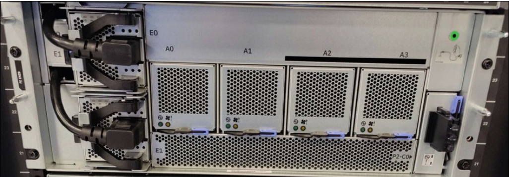
Figure 3-4 PCIe Gen 4I I/O expansion drawer front view
