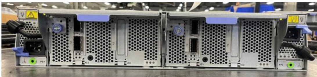
Figure 3-18 NED24 NVMe drawer rear view
