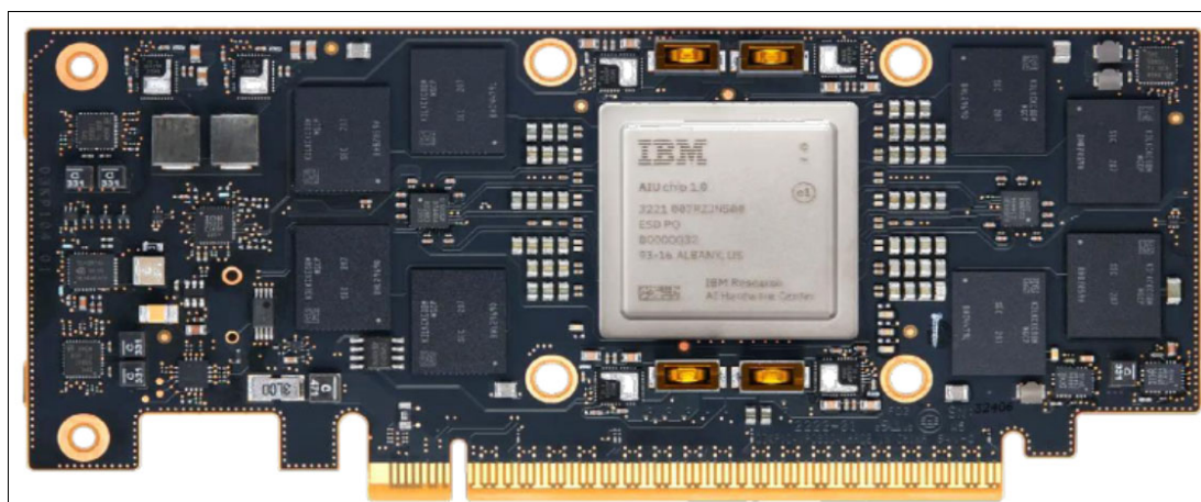
Figure 1-13 IBM Spyre Accelerator
