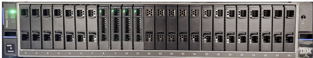
Figure 3-17 NED24 NVMe drawer front view
